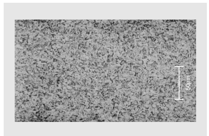
Fig. 1 - Microstructure of HCL307.
