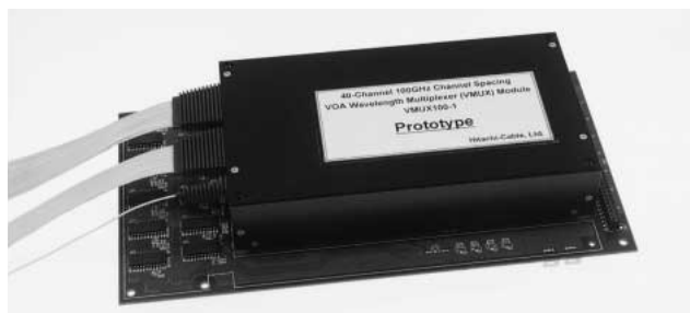
Fig. 9—Photograph of VOA-MUX module All optics are compactly mounted on the electrical circuits board.
